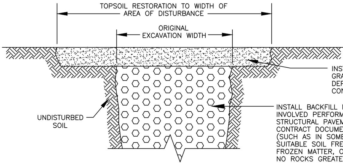
INSTALL 4" MINIMUM DEPTH OF TOPSOIL, MD S.H.A. MIX NO. 1 GRASS SEED, AND MULCH ALL IN ACCORDANCE WITH THE MD DEPT. OF TRANS. S.H.A. "STANDARD SPECIFICATIONS FOR CONSTRUCTION AND MATERIALS" SECTIONS 701-705.
