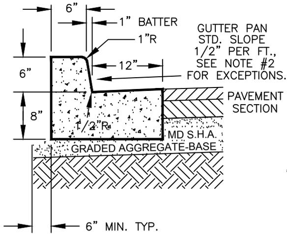
USE THIS CURB & GUTTER SECTION ON BOTH SIDES OF A MAJOR COLLECTOR, MINOR COLLECTOR, OR LOCAL STREET WHEN ON STREET PARKING IS PROPOSED ON ONE OR BOTH SIDES.
